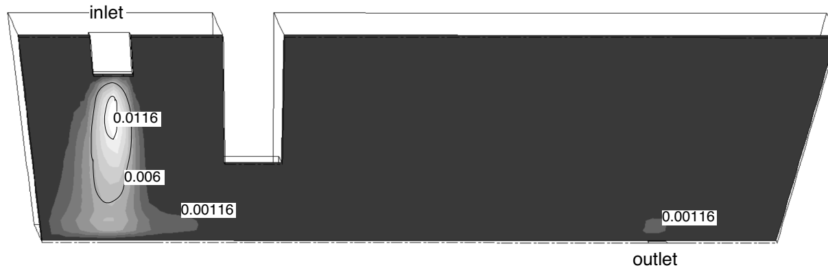
Figure 10 Distribution of kinetic energy on center plane ( \text{m}^2/\text{s}^2 ) (coupled flow-temperature model)
