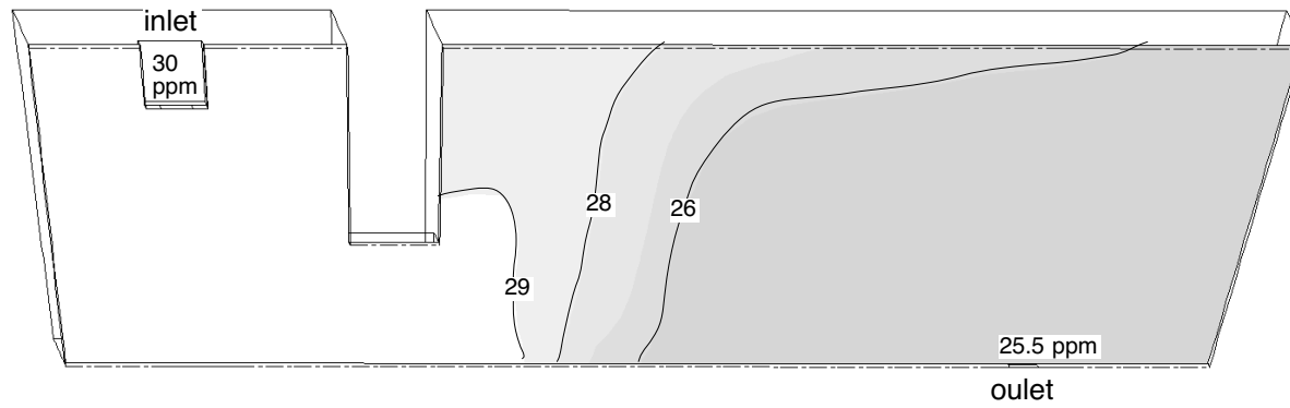
Figure 26 \text{Al}_2\text{O}_3 concentration at 1,000 sec
