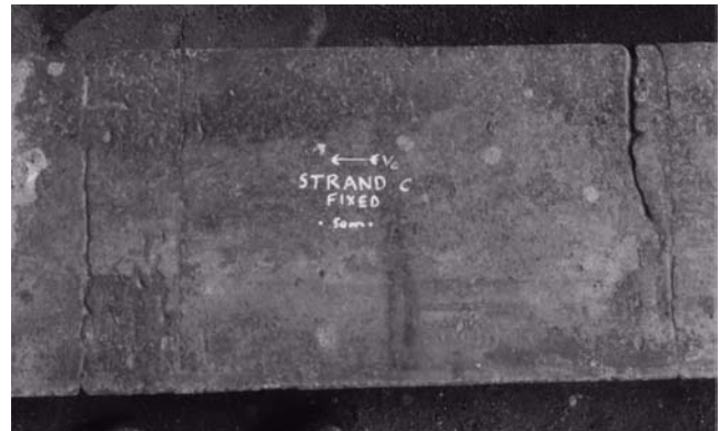
Fig. 1 Deep depression extending around the perimeter of the mold occurring during startup.
