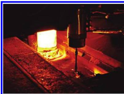
**1 Image of view of continuous casting mould from top (courtesy of Dr B. Stewart, Tata Steel)**
