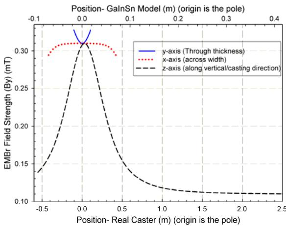
Fig. 3 Applied magnetic field in the x,y and z directions for GaInSn model and real caster.
