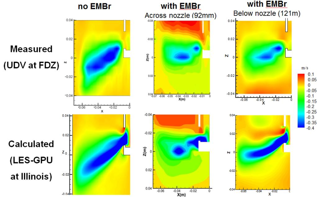
Fig. 5 Comparison of measured and simulated UDV signals
