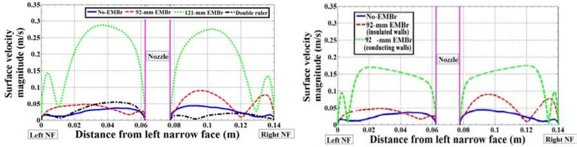
Fig. 8 Horizontal velocity profiles across top surface
