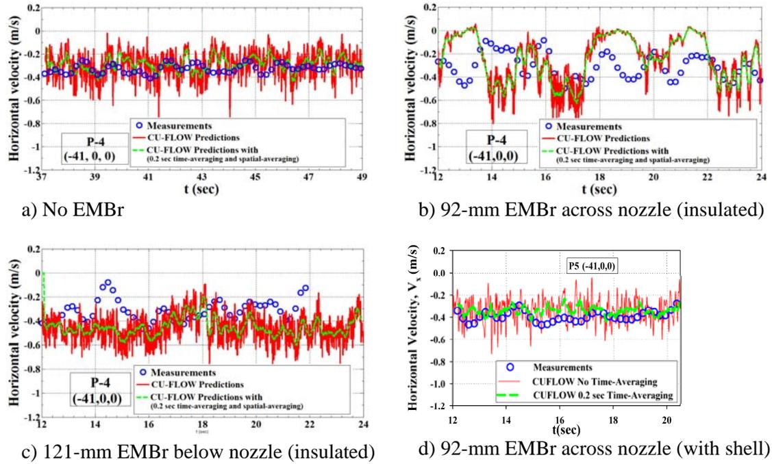
Fig. 6 Typical transient horizontal velocity, comparing predictions and measurements.
