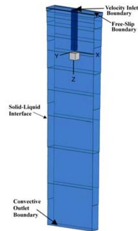
Fig. 4 Isometric view of computational flow domain (real caster).
