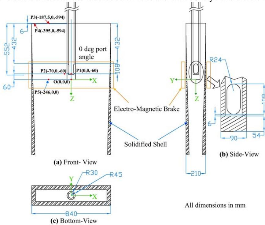
Fig.2 Geometry of the real caster with a rectangle showing the ruler EMBr location.
