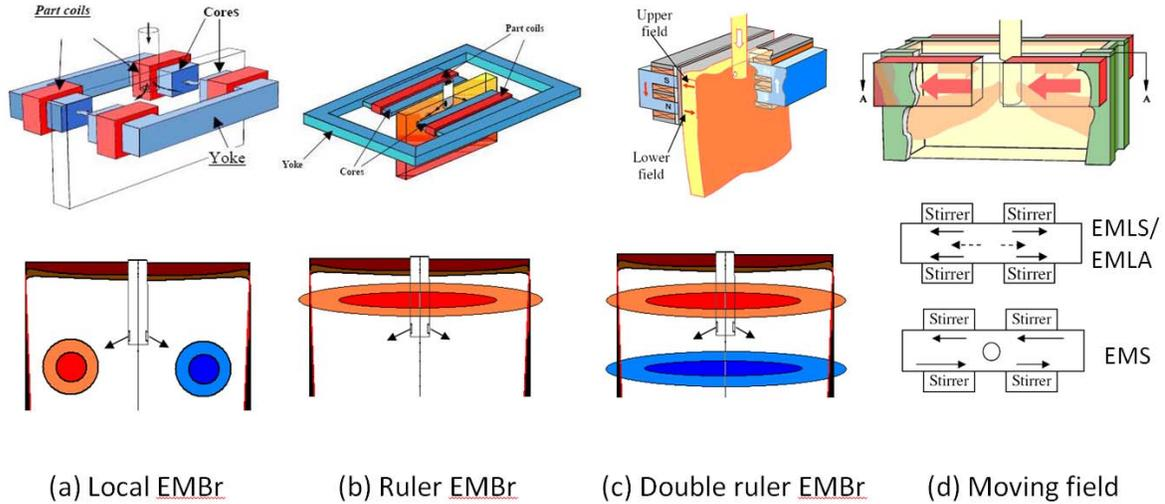
Fig.1 Types of electromagnetic flow control systems in slab casting showing magnet configuration (top) and magnetic field location (bottom)
