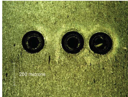
Figure 2. Several FBG sensors (200 \mu\text{m} diameter, plastic coated optical fibers) after electroplating with nickel
