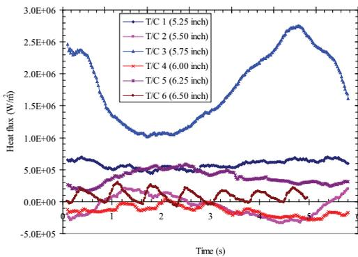
Fig. 11. Calculated heat flux histories on the mold surface (2-D inverse model)
