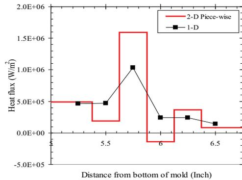
Fig. 12. Time-average heat flux profile down mold (z direction)
