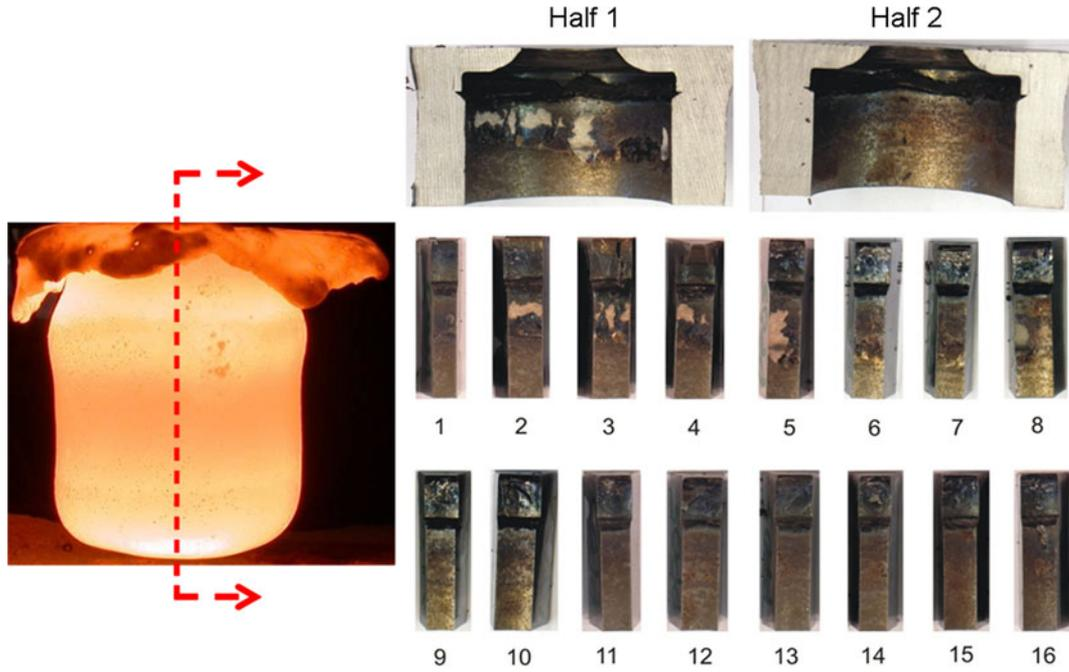
Fig. 3, Illustration of shell cutting for analysis.
