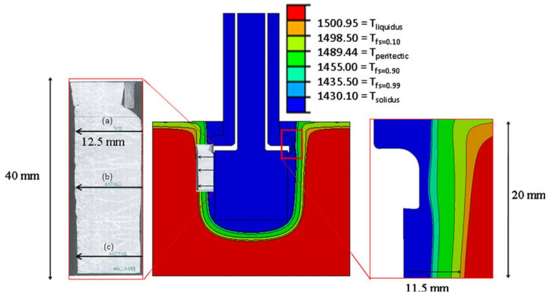
Fig. 9., Temperature contour at 25 s including shell and thickness measurement locations.
