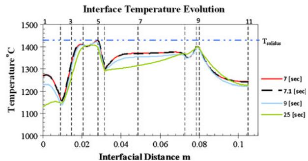
Fig. 8., Interface temperature for different simulation times.
