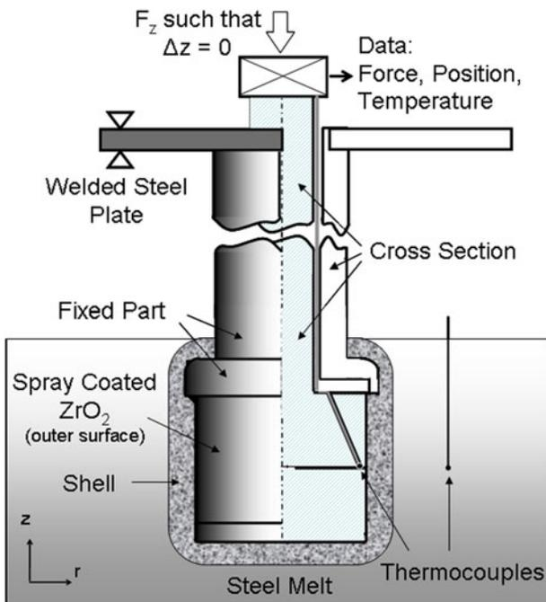
Fig. 2.,Schematic representation of the SSCC test.
