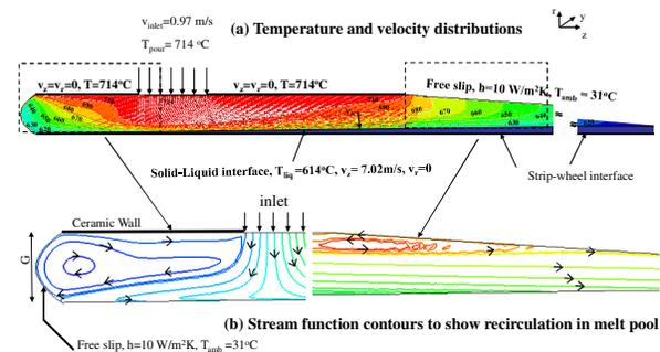
Fig. 3 Fluid flow model velocity and temperature distributions in the puddle region[5].
