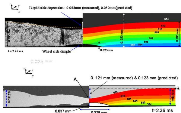
Fig. 2 Measured (left) versus predicted (right) transverse solidified shapes for (top) BN deposit and (bottom) air gap entrained during meniscus oscillation.
