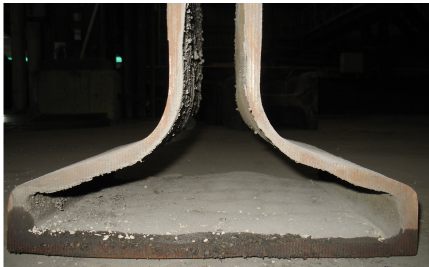
Figure 8. Photograph of Breakout Shell
