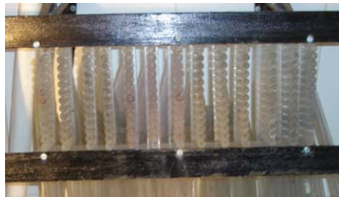
Fig. 3: Water collector used in the distribution measurements
