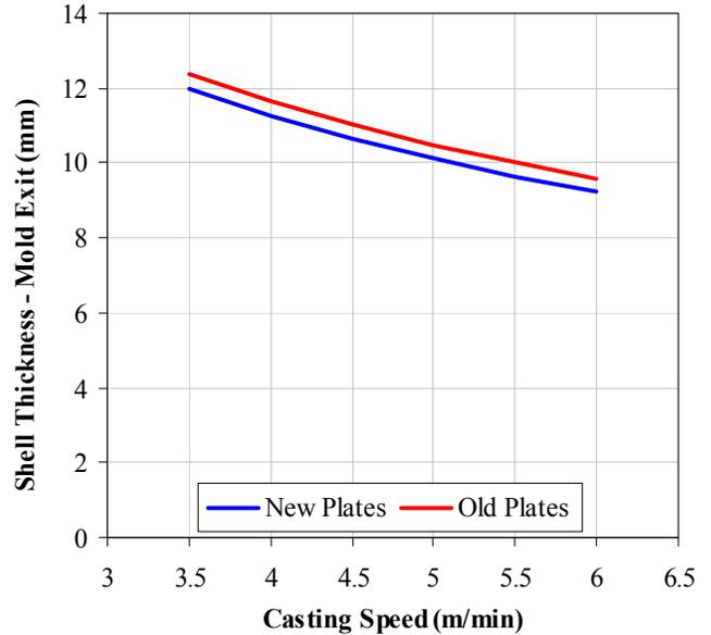
Figure 20. Effect of casting speed on shell thickness
