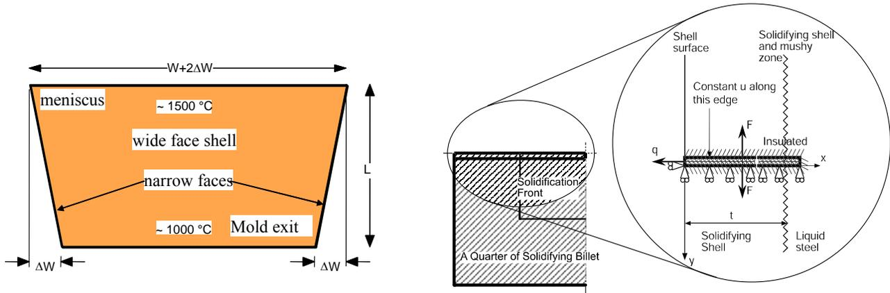
Fig. 1: Wide face shrinkage and narrow face taper Fig. 2: 1-D Slice Simulation Domain for CON2D
