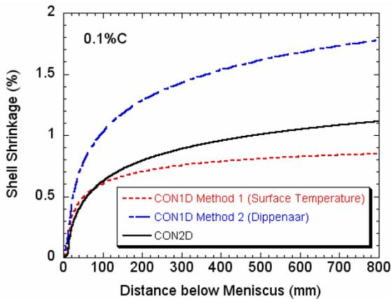
Fig. 13: Typical shrinkage profile comparison for low and medium-carbon steels (Powder E)
