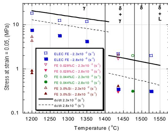
Fig. 4: Steel strength at high temperature (comparing predicted and measured values for  $\alpha$  and  $\gamma$ )
