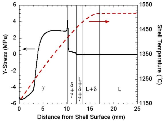
Fig. 11: Stress Profile through shell
