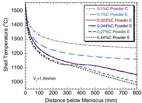
Fig. 10: Predicted surface temperature profiles
