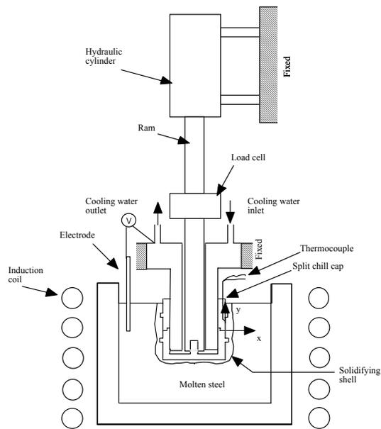
Fig. 5: Submerged Split Chill Tensile (SSCT) apparatus<sup>[1, 13]</sup>
