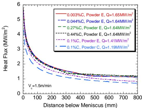
Fig. 9: Heat flux predicted down mold
