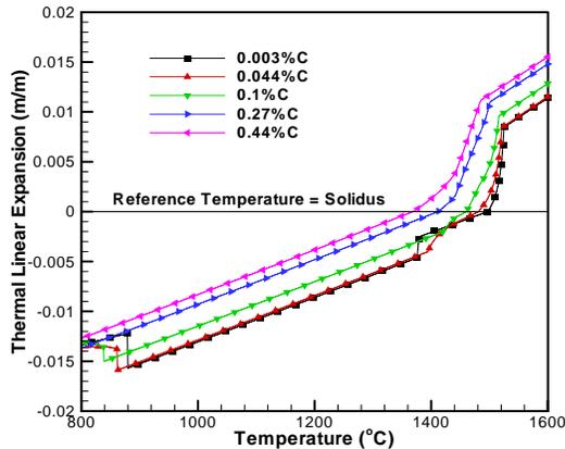
Fig. 3: Thermal expansion of steel,  $TLE(T)$
