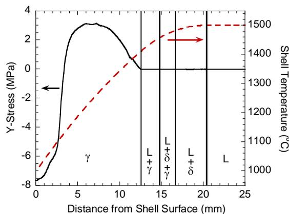
Fig. 7: Typical temperature and stress profiles predicted through shell thickness.
