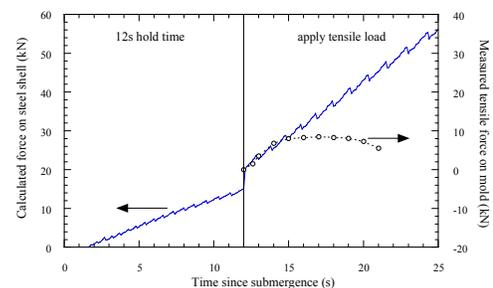
Fig. 8: Comparison of measured and simulated force during SSCT test
