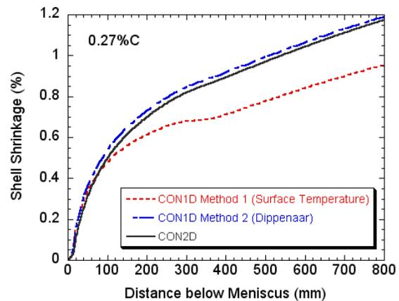
Fig. 14: Typical shrinkage profile comparison predicted for high-carbon steel
