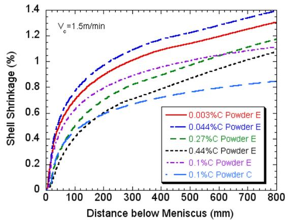
Fig. 12: CON2D Shrinkage predictions
