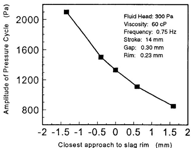
13 Effect of distance from mean slag rim position on slag pressure: slag consumption was reduced to zero as the rim entered the gap (closest approach to slag rim <0)
