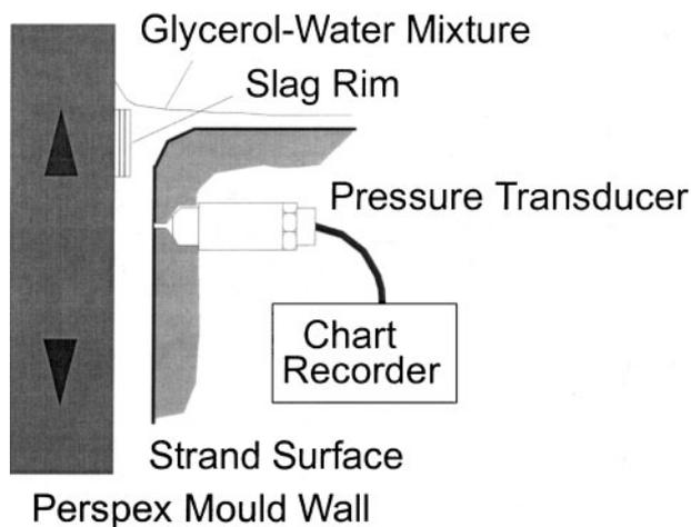
12 Schematic of physical model used to simulate meniscus region
