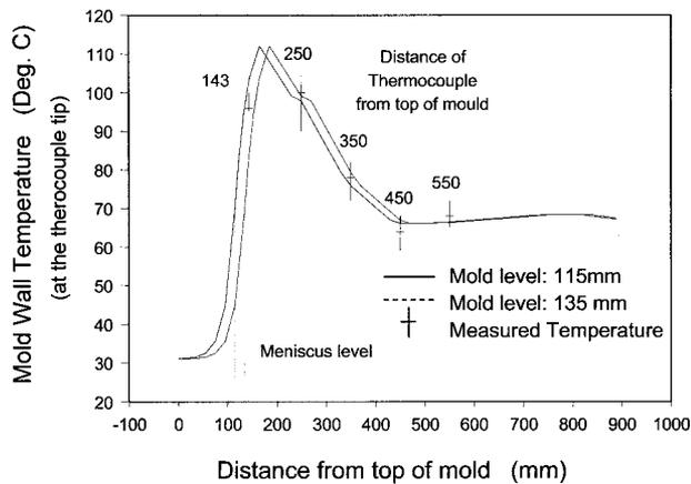
9 Predicted mould temperature profiles for a 20 mm change in mould level
