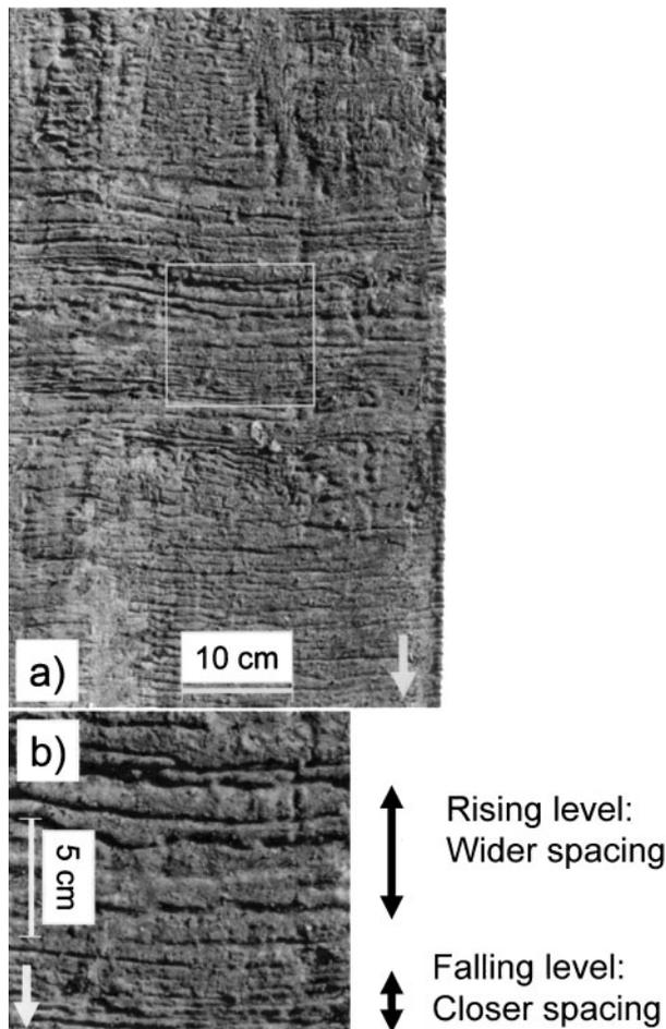
1 a variation in oscillation mark profile and pitch caused by gradual meniscus level variations and b close-up: arrow indicates casting direction
