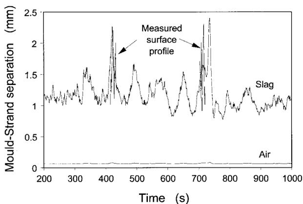
11 Predicted surface profiles for extreme cases of a completely slag and air filled mould-strand gap: a detailed measurement of the matching depressions has been shown for comparison; it is apparent the depressed regions must be almost entirely slag filled
