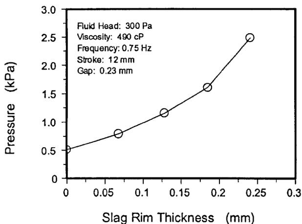
14 Effect of slag rim thickness on magnitude of pressure oscillation
