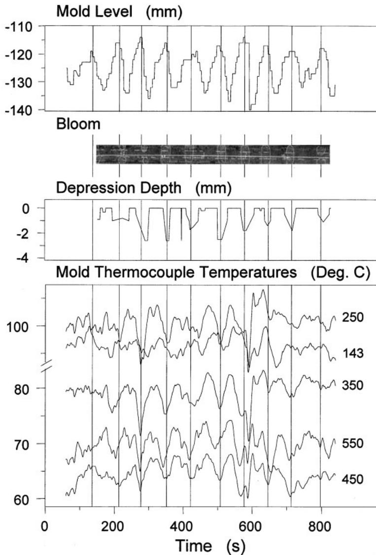
8 Photo of a bloom showing defects highlighted by chalked circles (centre) matched with the corresponding mould level history (top) and the thermocouple temperature profiles (bottom): the latter data has been shifted in time, according to casting speed and distance from the top of the mould, to the same reference point; the measured surface profile is also given (centre)
