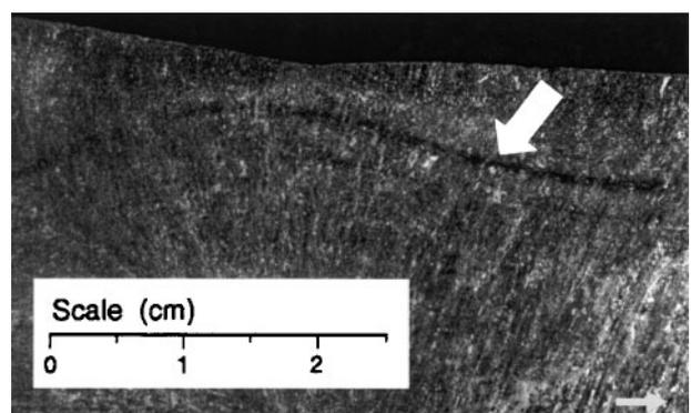
6 Sub-surface structure beneath a bloom depression: note the faint dark bands that indicate shell thinning as a result of the local reduction in cooling rate caused by the depression
