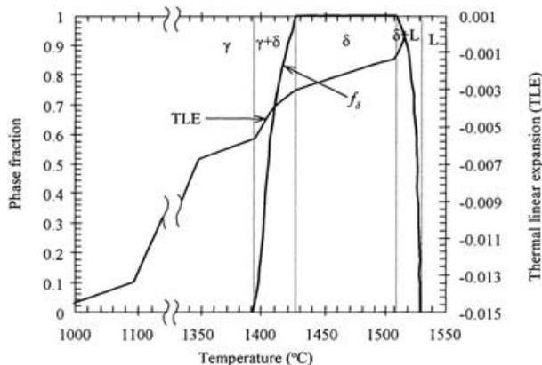
3 Calculated solid fraction  $f_s$ ,  $\delta$ -Fe fraction,  $\gamma$ -Fe fraction, and thermal linear expansion as function of temperature for low carbon (C = 0.04 wt-%) steel
