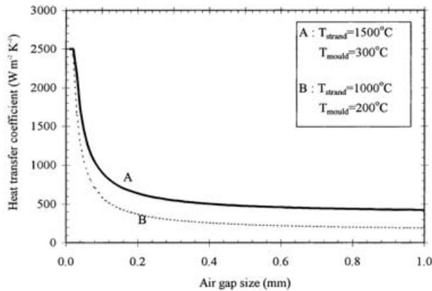
5 Heat transfer coefficient across strand/mould for various air gap sizes and given surface temperatures
