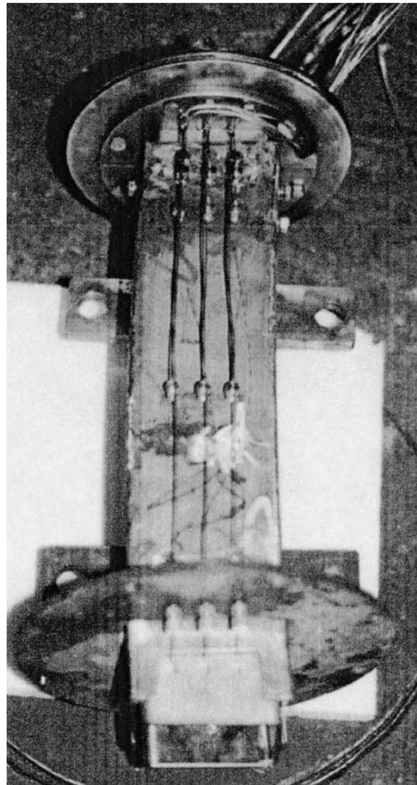
2 Photograph of thermocouple instrumented mould tube
