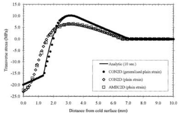
9 Comparison of calculated stress profiles with analytical solutions
