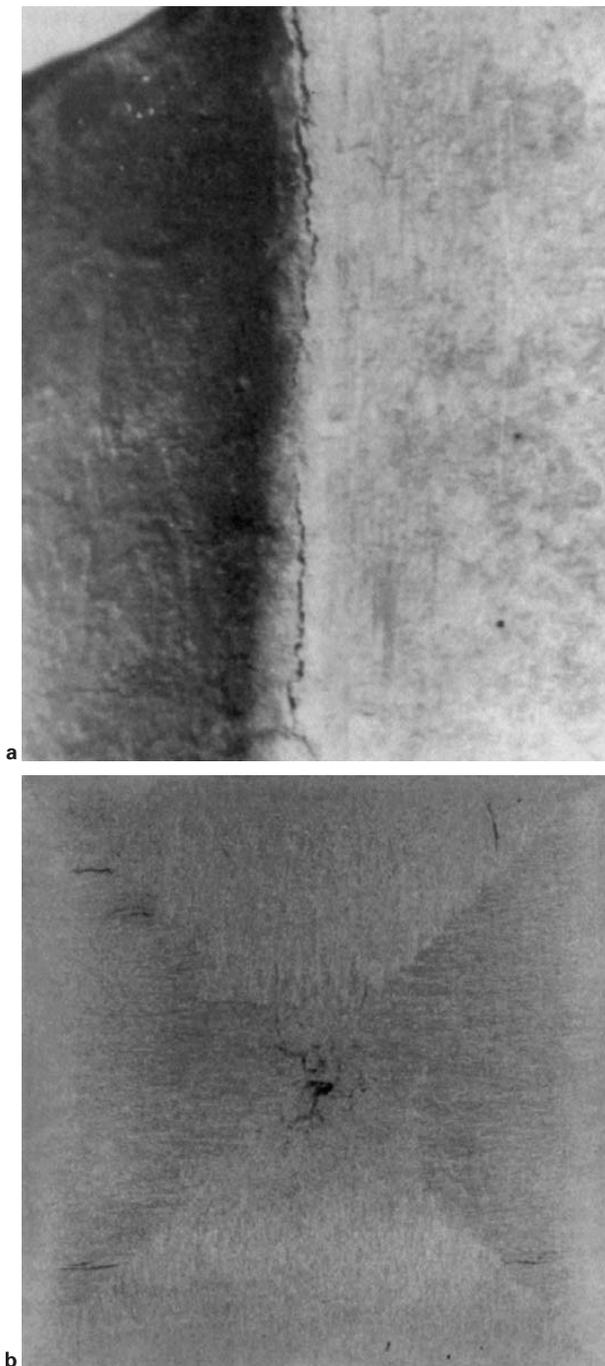
*a* longitudinal corner crack; *b* off corner internal cracks
