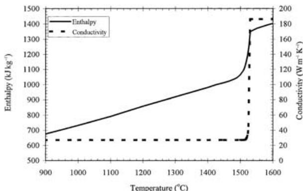
4 Enthalpy and conductivity of low carbon steel (C = 0.04 wt-%) used in present model
