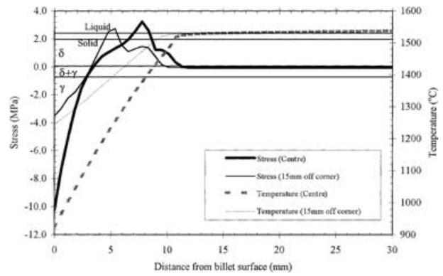
17 Temperature and transverse stress profiles through shell thickness at 19 s of casting time for 4 mm corner radius mould
