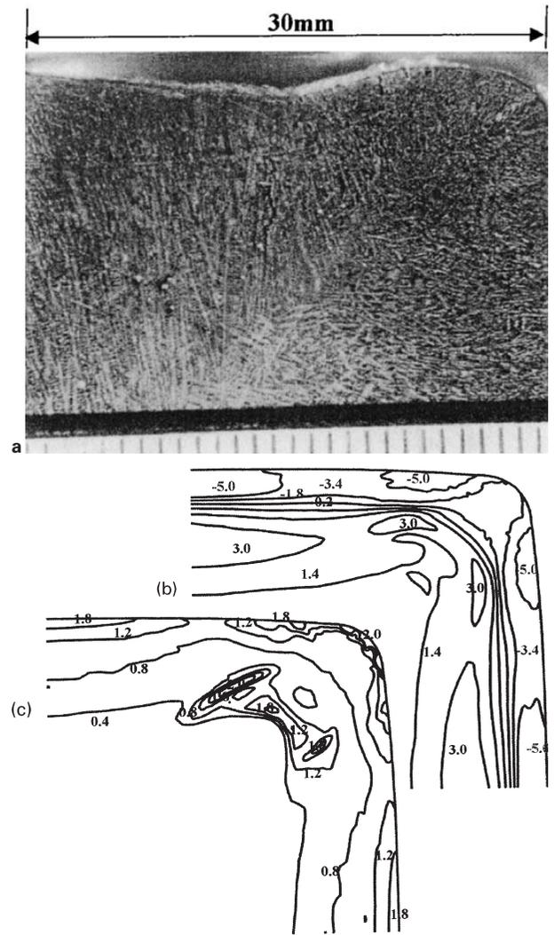
a microstructure of off corner crack; b hoop stress distribution; c equivalent plastic strain contours
