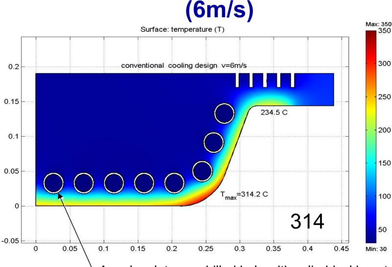
Annular slot: gun-drilled hole with cylindrical insert
