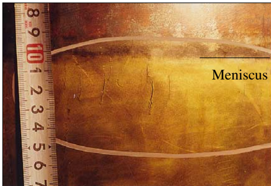
Fig. 28: Longitudinal cracks on hotface near meniscus of thin slab mold
